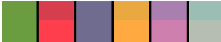
Red Gamma 1.5 Adjustment (Top) Compared to Color Compensation Filter Adjustment Matched on Third (Blue)
