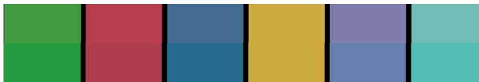
Red Gamma 0.667 Adjustment (Top) Compared to Color Compensation Filter Adjustment Matched on Fourth (Yellow)
